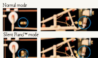
The Yamaha Quick Escape action automatically optimizes hammer escapement for normal and Silent Piano<sup>TM</sup> play, ensuring natural keyboard touch and response in either mode of play.
